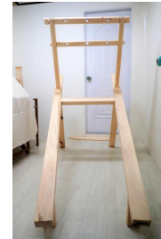
③ Assemble Legs and install Yongdumuri [용두머리]
