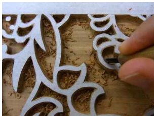
⑥ Refine it by using a chisel
