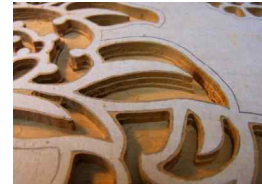
③ The same pattern is engraved three times with a depth of 0.3cm, 0.5cm, and 0.8cm
