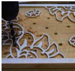
⑦ Punch holes for the dye
