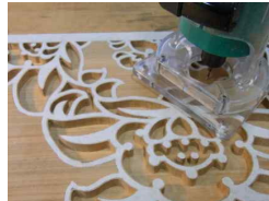
② Engrave the pattern with a trimmer
