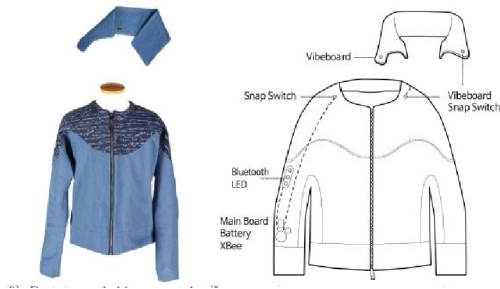
〈Fig. 6〉 Appearance and system embedding structure of type A (Im, Kim & Lee, 2016, p. 73)
