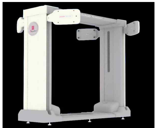
<Fig. 1> 3D Body Scanner 'Medi CUBE' (buyKOREA [3D Whole Body Scanner MEDICUBE] (2018, April 10). Retrieved from http://www.buykorea.org/product-details/3D-Whole-Body-Scanner-MEDICUBE-3007486.html )
